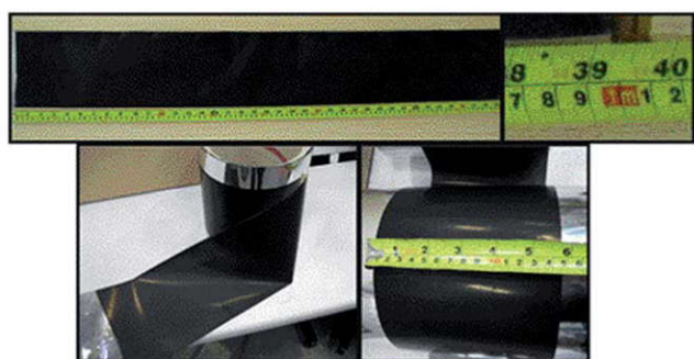
Fig. 9 Optical images of spray deposited CNT thin film on PET webs.
